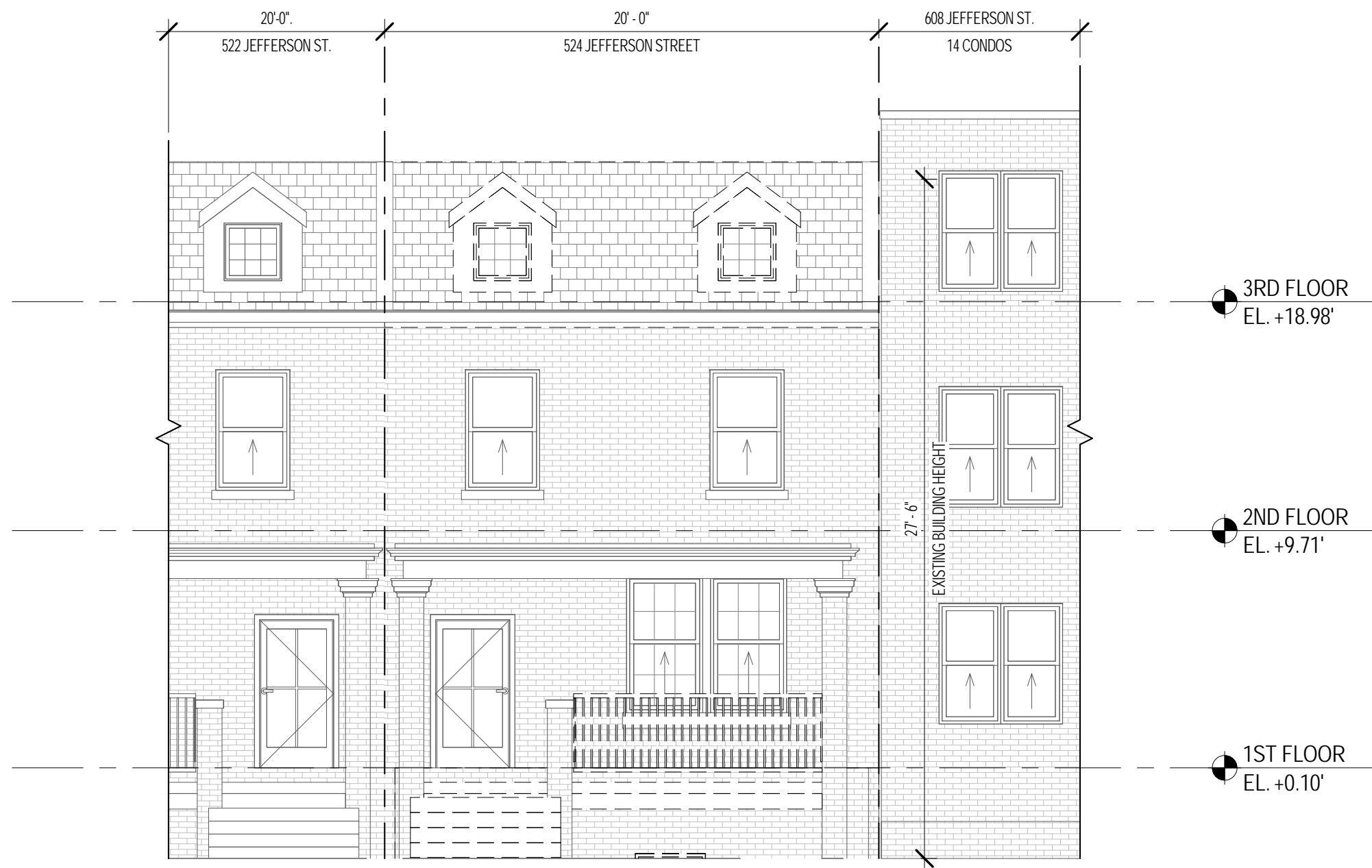
1 FRONT ELEVATION - EXISTING A007 3/16" = 1'-0"
